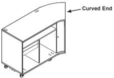
Right curved unit assembly shown **Lower Lock** Door (22)Hole for chamber lock is offset toward the curved end of the unit assembly Outside Surface Hole for Chamber Lock Assembly **Lower Lock** 1/4-20 x .787" **Door Plate Hex Socket** Outside (23)**Machine Screw** Surface (29)Clearance Holes **Bottom Edge** Q Q **Lower Lock** Clearance Door Hole (24)1/4-20 **Insert Nut** (5) Lower Lock **Door Plate** (23)
