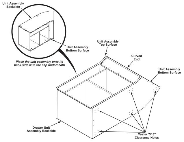
Right curved unit assembly shown with the backside resting on the floor (cap)
